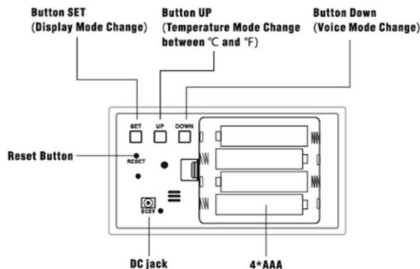
De instellingsstroom is: YEAR - MONTH - DATE - 12/24 HOURS - HOUR - MINUTE - ALARM 1 ON/OFF - ALARM HOUR - ALARM MINUTE - ALARM2 ON/OFF - ALARM2 HOUR - ALARM2 MINUTE - ALARM3 ON/OFF - ALARM3 HOUR - ALARM3 MINUTE - WORK DAY ALARM ON/OFF - EXIT
