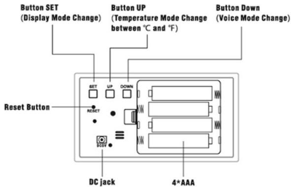
The setting flow is: YEAR - MONTH - DATE - 12/24 HOURS - HOUR - MINUTE - ALARM 1 ON/OFF - ALARM HOUR - ALARM MINUTE - ALARM2 ON/OFF - ALARM2 HOUR - ALARM2 MINUTE - ALARM3 ON/OFF - ALARM3 HOUR - ALARM3 MINUTE - WORK DAY ALARM ON/OFF - EXIT
